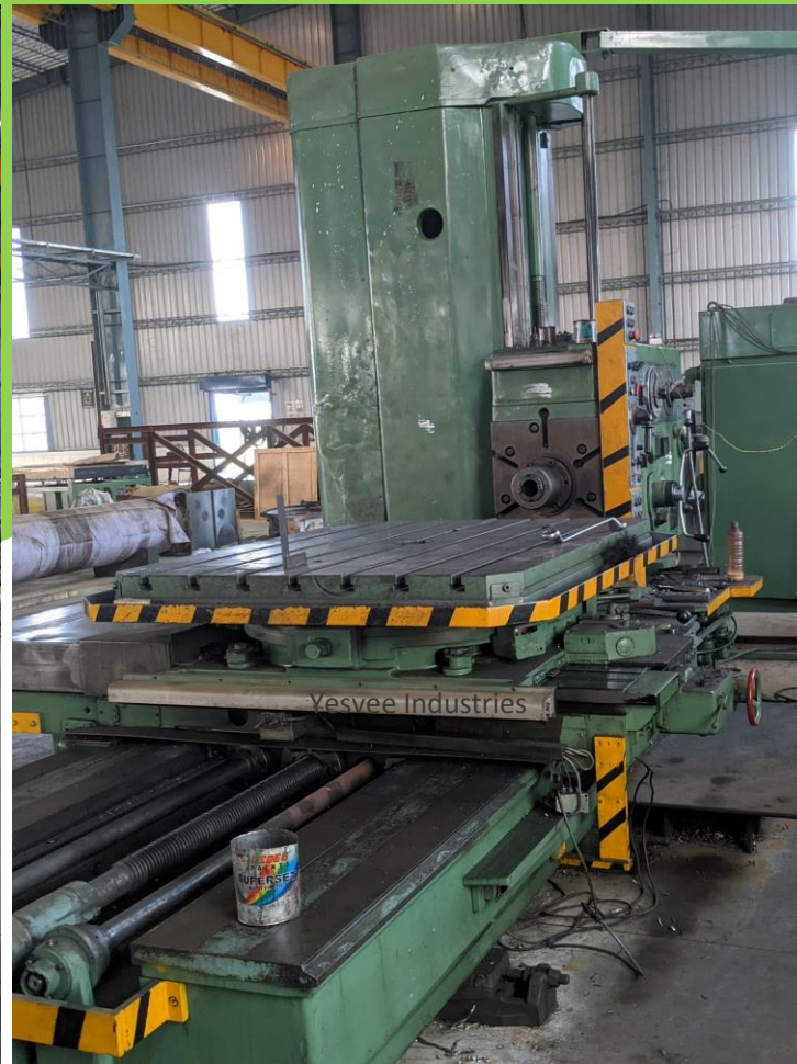
SPINDLE- 125 MM DIA 800 MM TRAVEL
